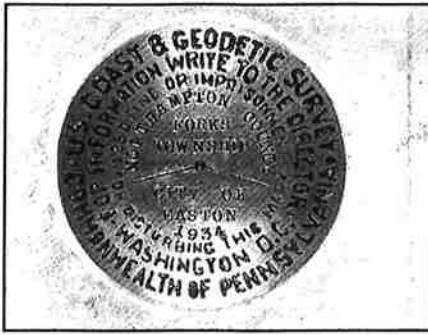
Survey mark set by a public works agency party in Pennsylvania for boundary survey and bench mark, February 19, 1934. More than 10,000 unemployed surveyors, engineers, and technicians participated in the surveys nationwide.
